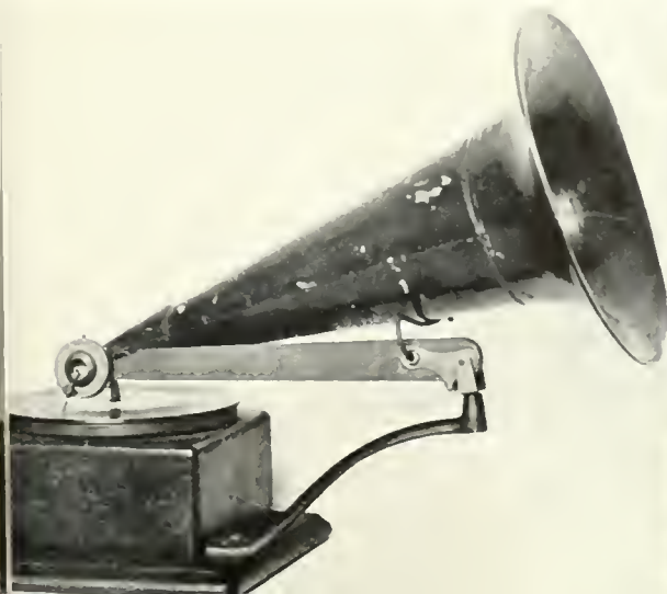
THE BERLINER GRAMAPHONE, PATENTED IN 1887, FEATURED A FLAT DISC AND A HORN, IN CONTRAST TO THE CYLINDRICAL RECORDS THEN IN COMMON USE.
