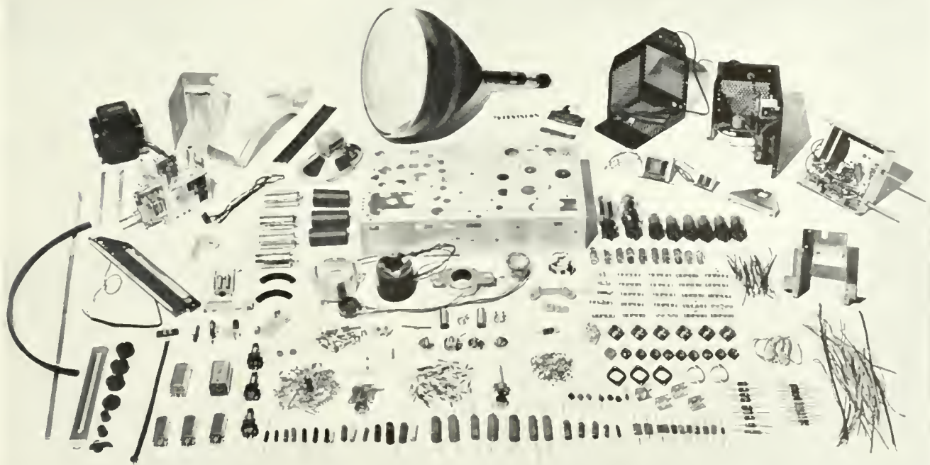
SOME OF THE HUNDREDS OF PARTS AND SUB-ASSEMBLIES THAT GO INTO THE MAKING OF A 12½-INCH TELEVISION RECEIVER.
