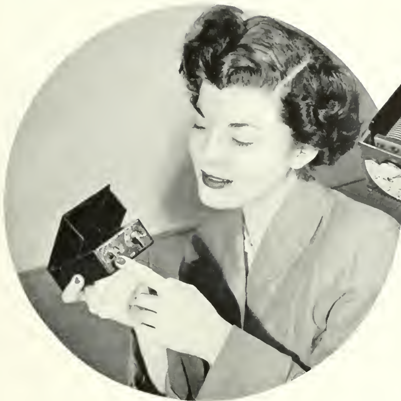
CONTAINING FOUR MINIATURE TUBES AND ALL BATTERIES, THE RECEIVER IS SMALL ENOUGH TO FIT EASILY INTO A POCKET OR MILADY'S HANDBAG. BELOW: COMPARISON OF PREVIOUS "PERSONAL" RADIO AND THE LATEST MODEL.
