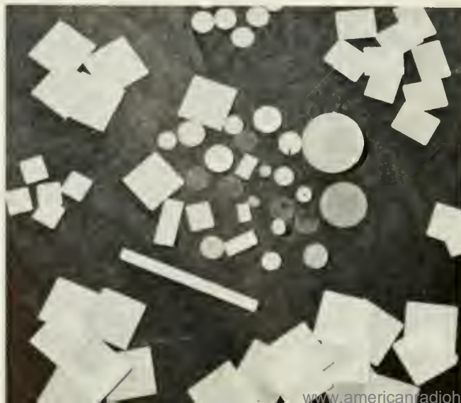
SOME OF THE MANY TYPES OF QUARTZ CRYSTALS PRODUCED BY RCA FOR THE CONTROL OF RADIO FREQUENCIES.
